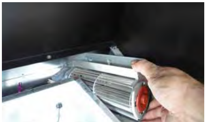
Figure 31. Sliding the blower into place.
