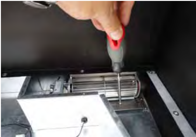
Figure 32. Location of blower mounting screws.
