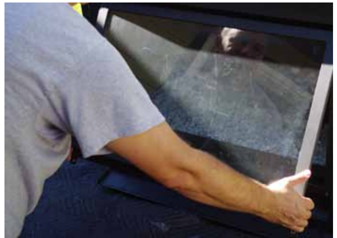
Figure 24. Remove Door by grabbing both sides of the frame, Lifting up, pull the Door away from fireplace. Store the Door in a safe place where it will not get damaged. Replace in reverse order.
