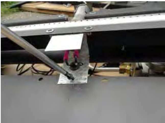
Figure 33. Mounting the thermal switch.
