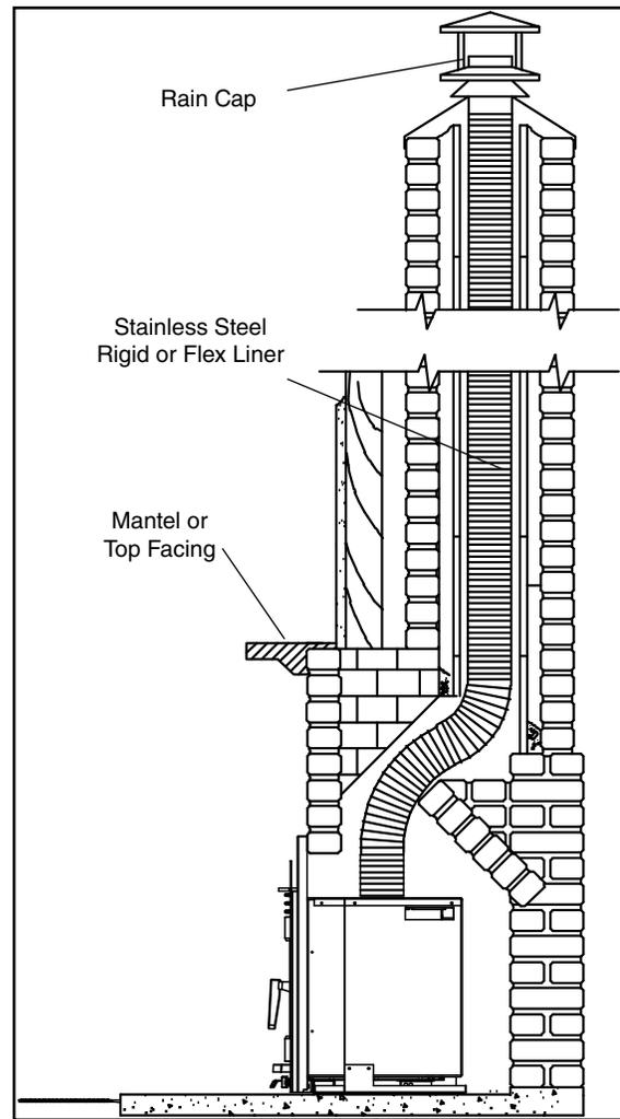
**Pacific Energy highly recommends the use of a full liner as the safest installation and providing optimum performance. When connected to a full liner, the Insert is able to draft correctly and will prevent problems such as difficult start-ups and smoking out the door.**
