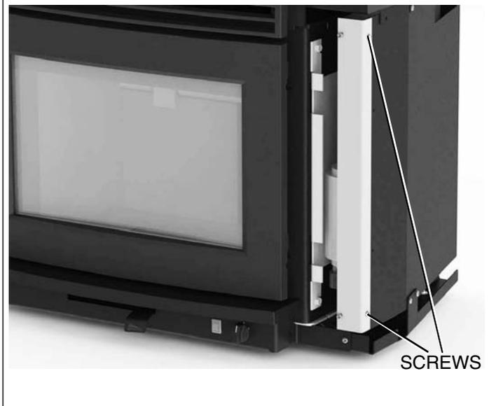
3. With a 3/8" wrench, loosen the two bolts securing the blower mounting bracket to the unit. Fig. #3
